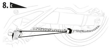
**EN** Tighten the cord by sliding the RIDER and checking its positioning so that it does not touch other parts of the motorcycle. The minimum distance from the sprockets is 100mm (4in). The angle between the cord and the chain must not be greater than 45 degrees.
