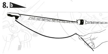
**EN** Thread the cord through the bottom hook so that the knot is down just below the hook. Cut the excess cord 5mm (0.2in) below the knot.
