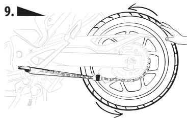
**EN** Turn the wheel in the direction of the arrows until the entire chain passes through the RIDER. If the motorcycle is not standing on a central or service stand, gently push the motorcycle forward approximately 7m (23ft) until the entire chain passes through the RIDER.
