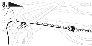
**EN** Loop the cord around the footpeg or other fixed point of the motorcycle in the direction of the front of the motorcycle and proceed to the bottom hook of the RIDER.
